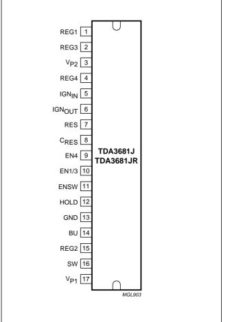
Fig.3 Pin configuration for TDA3681J and TDA3681JR.
