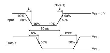
Note 1: Pulse Width 50  $\mu s$ , Duty Cycle 10%
