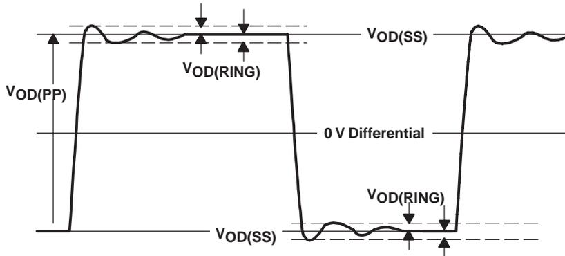
NOTE:  $V_{OD(RING)}$  is measured at four points on the output waveform, corresponding to overshoot and undershoot from the  $V_{OD(H)}$  and  $V_{OD(L)}$  steady state values.
