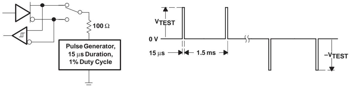
Figure 16. Test Circuit and Waveforms, Transient Overvoltage Test
