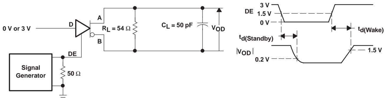
Figure 8. Driver Standby/Wake Test Circuit and Waveforms
