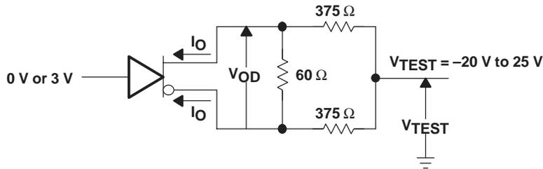
Figure 2. Driver Test Circuit,  $V_{OD}$  With Common-Mode Loading
