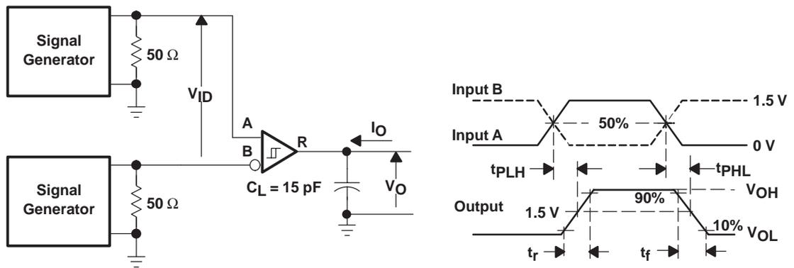
Figure 11. Receiver Switching Test Circuit and Waveforms
