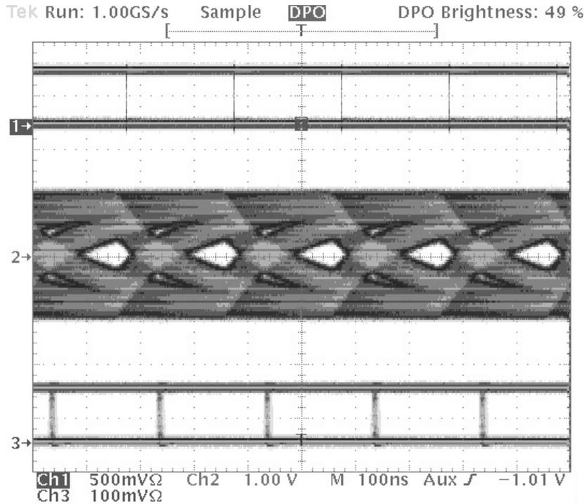
Figure 28. HVD24 Receiver Performance at 5 Mbps Over 500 Meter Cable
