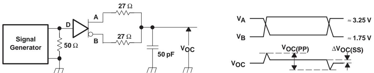
Figure 4. Driver  $V_{OC}$  Test Circuit and Waveforms
