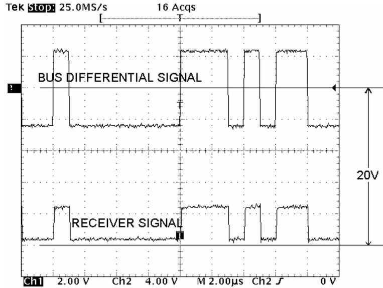
Figure 25. HVD22 Receiver Operation With 20 V Offset on Input Signal
