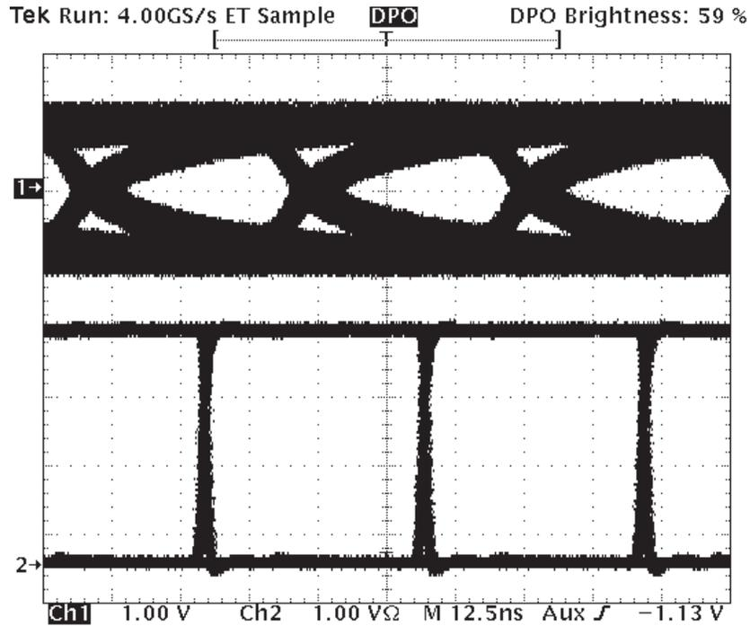
Figure 27. HVD23 Receiver Performance at 25 Mbps Over 150 Meter Cable
