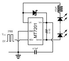
The amplitude of PWM signal need to be larger than 2.0V, normally  $3.0V \sim 5V$ . The frequency of the PWM dimming signal better to be  $100Hz \sim 2KHz$ .
