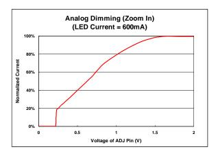
voltage (VADJ), as shown, to adjust the output current to a value below the nominal average value defined by Rs.
