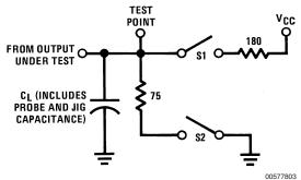
S1 and S2 of load circuit are closed except where shown.
