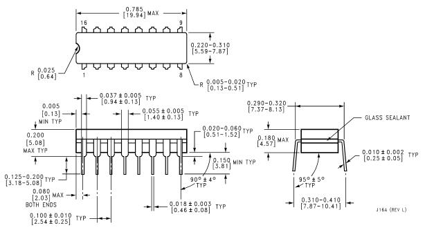
16 Lead Ceramic Dual-in-Line Package (J)
