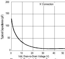
**Figure 2. Typical Output Capacitance**
