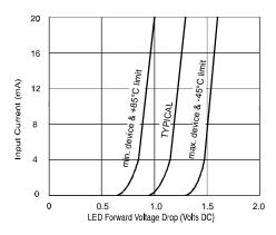
Figure 6. Input Characteristics (Current Controlled)
