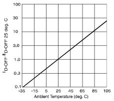
Figure 5. Typical Normalized Off-State Leakage
