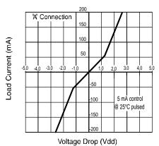
Figure 3. Linearity Characteristics
