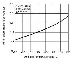
Figure 4. Typical Normalized On-Resistance
