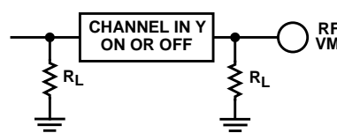
FIGURE 22. CROSSTALK BETWEEN DUALS OR TRIPLETS (CD4052B, CD4053B)
