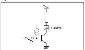
This output stage is intended for "reverse" base control, where setting the output NPN in off-state will control the power scanning transistor in off-state (see Application Diagram).
