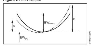
Figure 4: Keystone Effect on E/W Output (PCC Inhibited)
