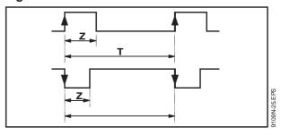
Using internal integration, both signals are recognized if Z/T < 25%. Synchronization occurs on the leading edge of the internal sync signal. The minimum value of Z is  $0.7\mu s$ .
