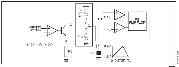
The syncfrequency must always be higher than the free running frequency. For example, when using a sync range between 24kHz and 100kHz, the suggested free running frequency is 23kHz.
