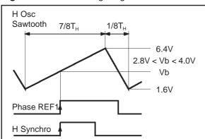
Phase REF1 is obtained by comparison between the sawtooth and a DC voltage adjustable between 2.8V and 4.0V. The PLL1 ensures the exact coincidence between the signal phase REF and HSYNC. A  $\pm$  T<sub>H</sub>/10 phase adjustment is possible.
