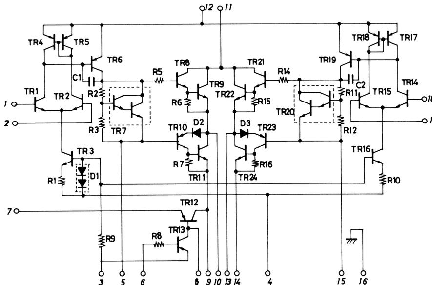
Sample Application Circuit : 50W min AF Power Amplifier (2 channels)
