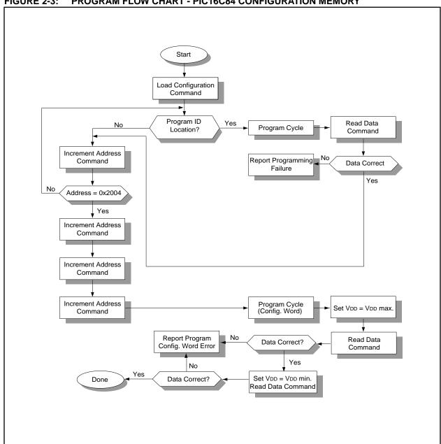
FIGURE 2-3: PROGRAM FLOW CHART - PIC16C84 CONFIGURATION MEMORY
