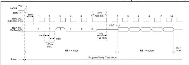
FIGURE 5-3: INCREMENT ADDRESS COMMAND (SERIAL PROGRAM/VERIFY)
