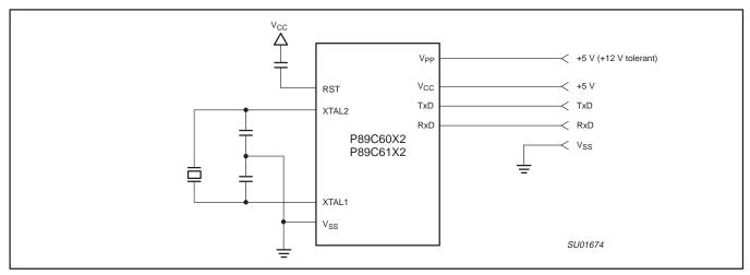
Figure 2. In-System Programming with a Minimum of Pins
