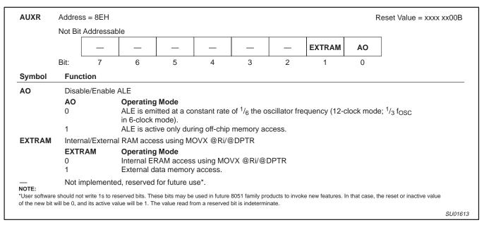
Figure 29. AUXR: Auxiliary Register
