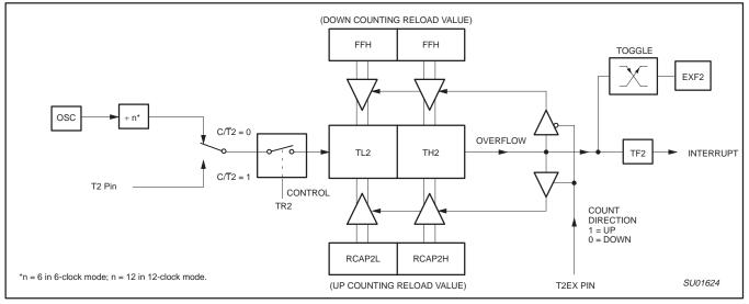
Figure 12. Timer 2 Auto Reload Mode (DCEN = 1)
