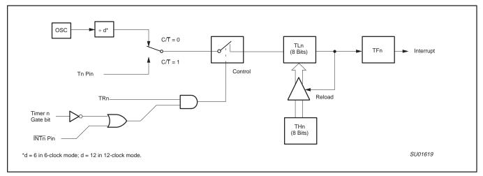
Figure 6. Timer/Counter 0/1 Mode 2: 8-Bit Auto-Reload
