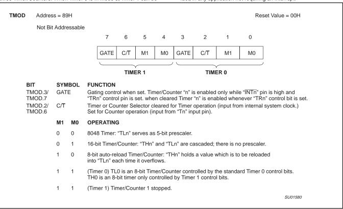
Figure 3. Timer/Counter 0/1 Mode Control (TMOD) Register
