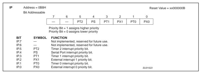
Figure 25. Interrupt Priority (IP) Register
