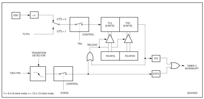
Figure 11. Timer 2 in Auto-Reload Mode (DCEN = 0)
