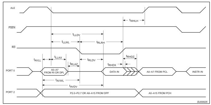
Figure 32. External Data Memory Read Cycle
