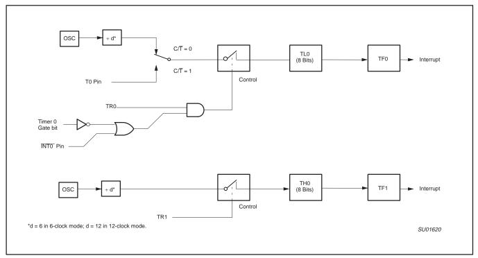
Figure 7. Timer/Counter 0 Mode 3: Two 8-Bit Counters
