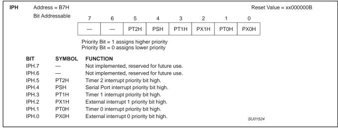
Figure 26. Interrupt Priority HIGH (IPH) Register
