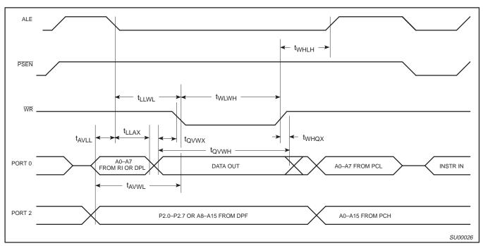
Figure 33. External Data Memory Write Cycle
