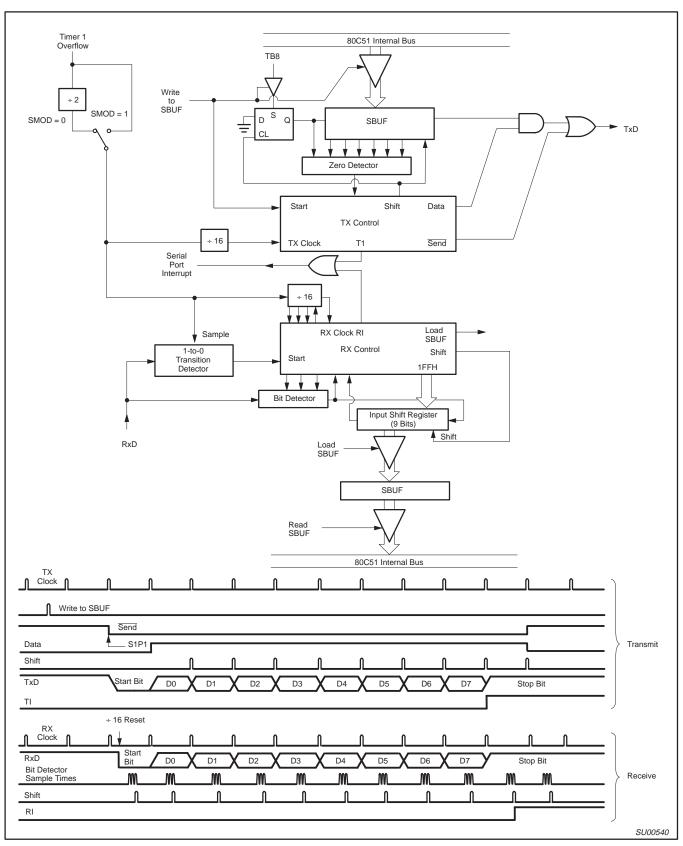
Figure 17. Serial Port Mode 1
