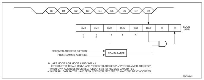
Figure 22. UART Multiprocessor Communication, Automatic Address Recognition
