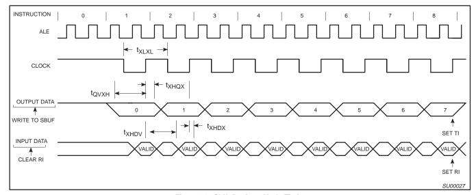
Figure 34. Shift Register Mode Timing
