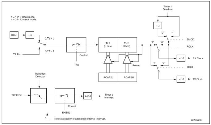
Figure 13. Timer 2 in Baud Rate Generator Mode
