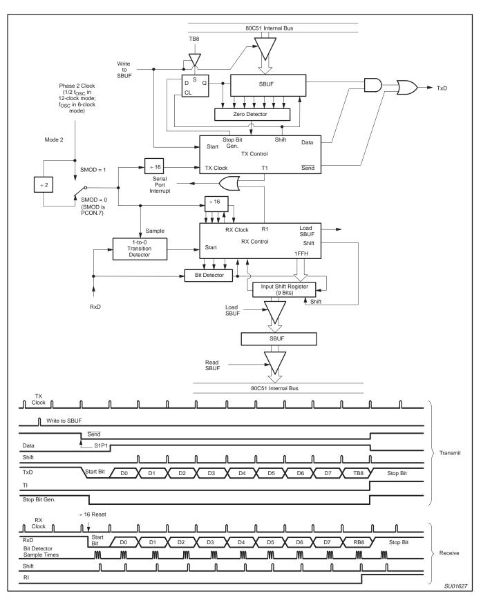
Figure 18. Serial Port Mode 2
