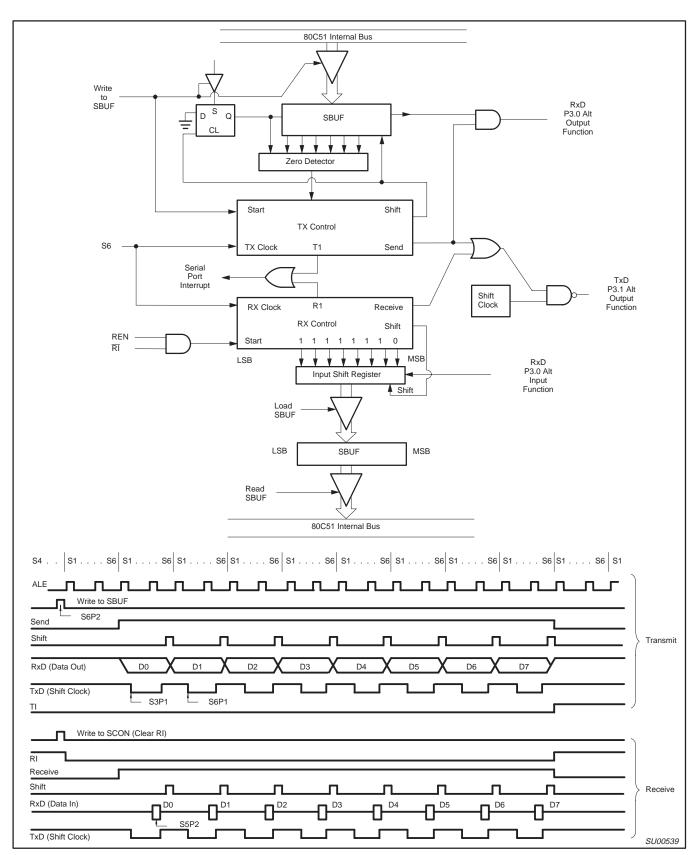
Figure 16. Serial Port Mode 0
