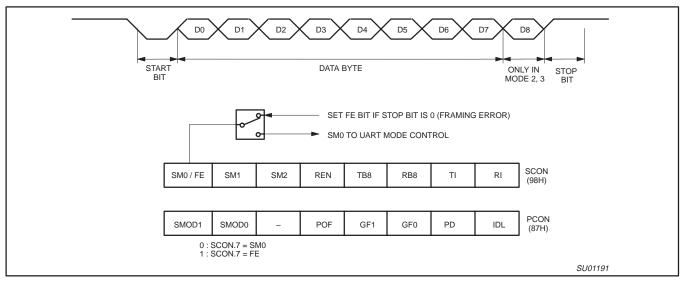
Figure 21. UART Framing Error Detection
