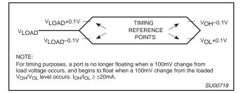
Figure 37. Float Waveform
