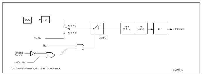
Figure 4. Timer/Counter 0/1 Mode 0: 13-Bit Timer/Counter
