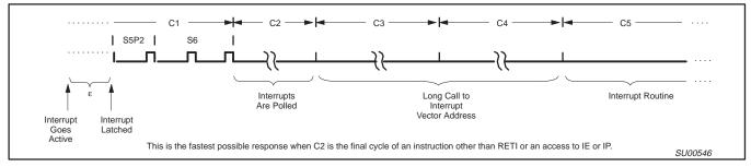
Figure 27. Interrupt Response Timing Diagram
