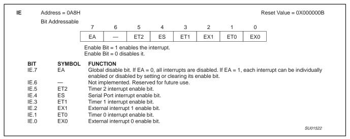
Figure 24. Interrupt Enable (IE) Register
