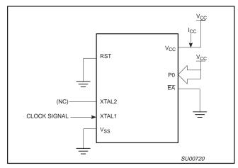
Figure 40. I<sub>CC</sub> Test Condition, Idle Mode All other pins are disconnected
