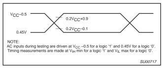
Figure 36. AC Testing Input/Output
