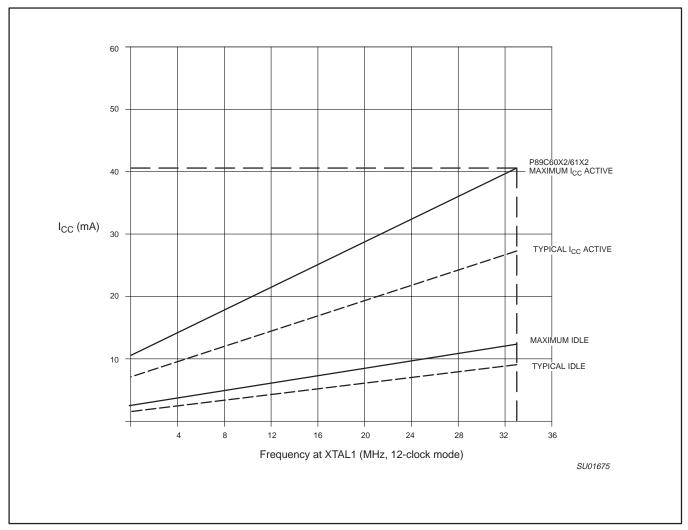
Figure 38. I<sub>CC</sub> vs. FREQ for 12-clock operation Valid only within frequency specifications
