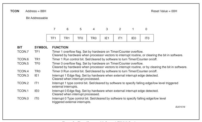
Figure 5. Timer/Counter 0/1 Control (TCON) Register
