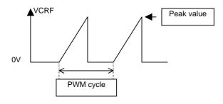
Caution: For the VCRF voltage of control characteristics, the peak value is to be measured. Cautions for use)
