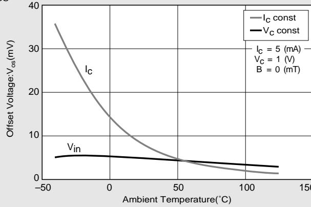
$V_{os}$ - $V_C$ ,  $V_{os}$ - $I_C$
