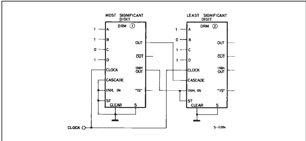
In the ADD mode some of the gaps left by the more significant unit at the count of 15 are filled in by the less significant units. For example, when two units are cascaded in the ADD mode and programmed to 11 and 13, respectively, the more significant unit will have 11 output pulses and the other unit will have 13 output pulses for every 256 input pulses for a total of :
