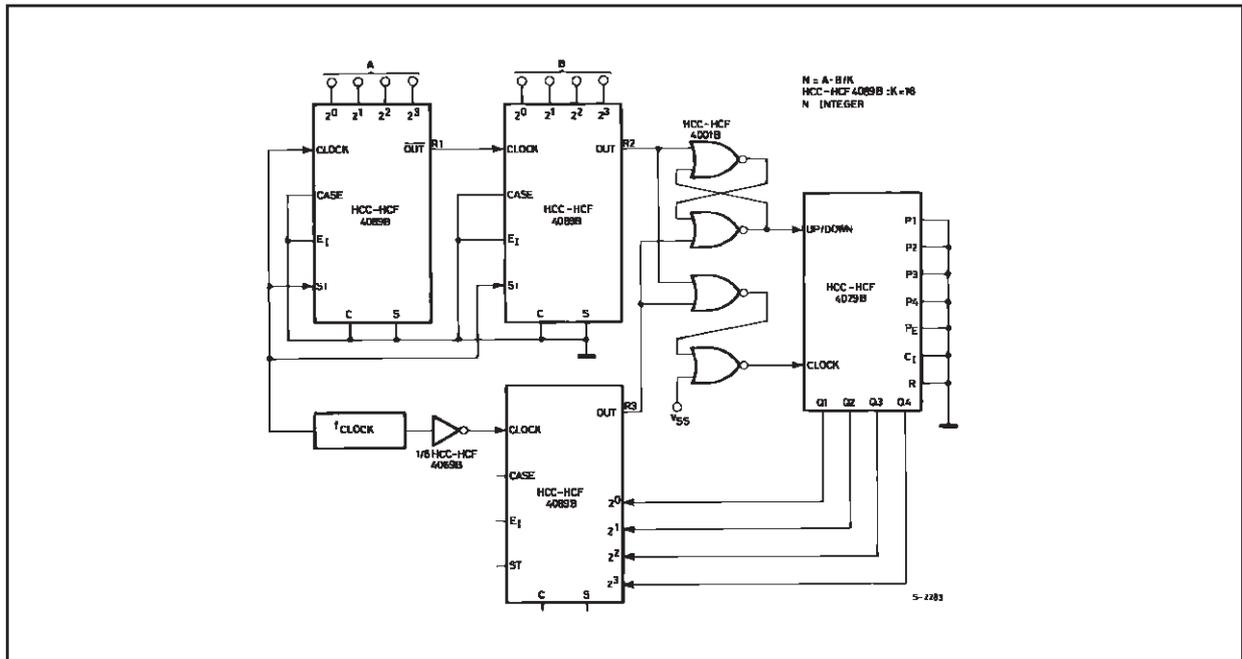
When the loop stabilities rate  $R2 = rate R3$ , thus  $f_{clock}(\frac{A}{16} \cdot \frac{B}{16}) = f_{clock}(\frac{1}{16} \cdot \frac{N}{16})$  therefore  $N = AB$
