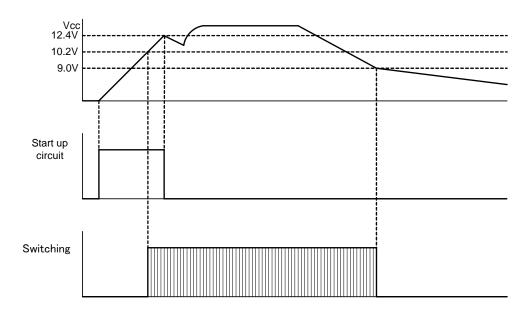
Fig.5 Startup and shutdown (the auxiliary winding voltage is higher than 10.2 V)
