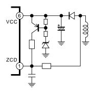
Fig.14 Primary side over voltage protection circuit
