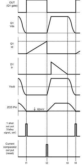
Fig.2 Waveform in basic operation
