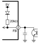
Fig. 15 FB pin circuit
