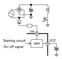
Fig.23 VH pin circuit (2)
