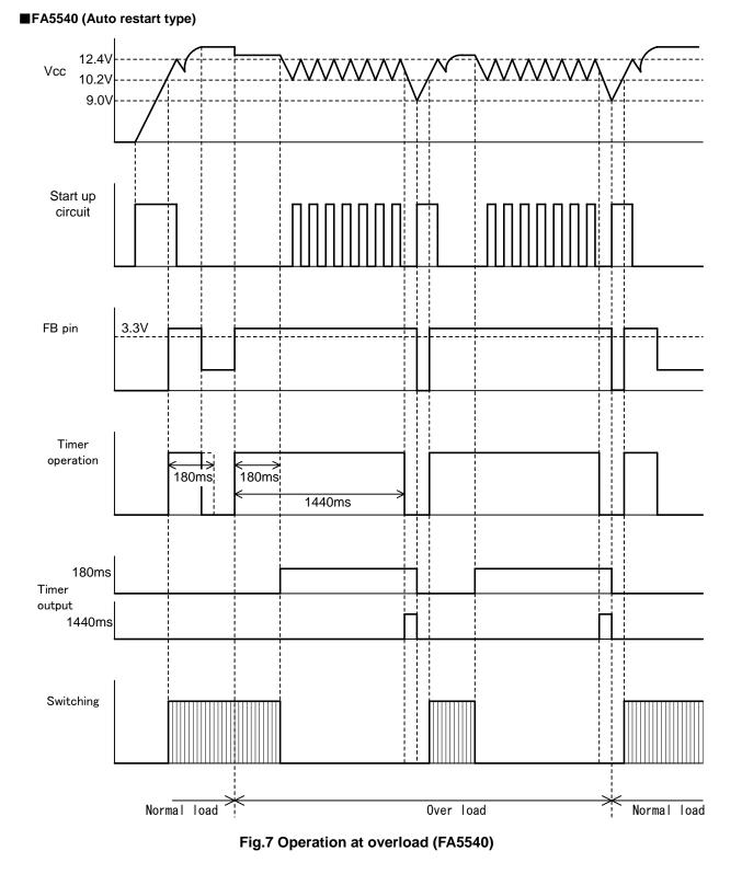
If an overload condition continues more than 180ms, switching is forced to shutdown using an internal timer. In addition the startup circuit is possible to operate within 1440ms from beginning of an overload condition. If an overload condition continues, switching is done for 180ms and after that Vcc is provided by a startup circuit for 1260ms and the operation halt condition is maintained.
