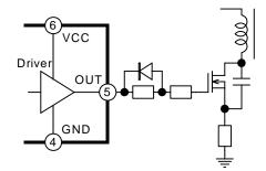
Fig. 19 OUT pin circuit (2)
