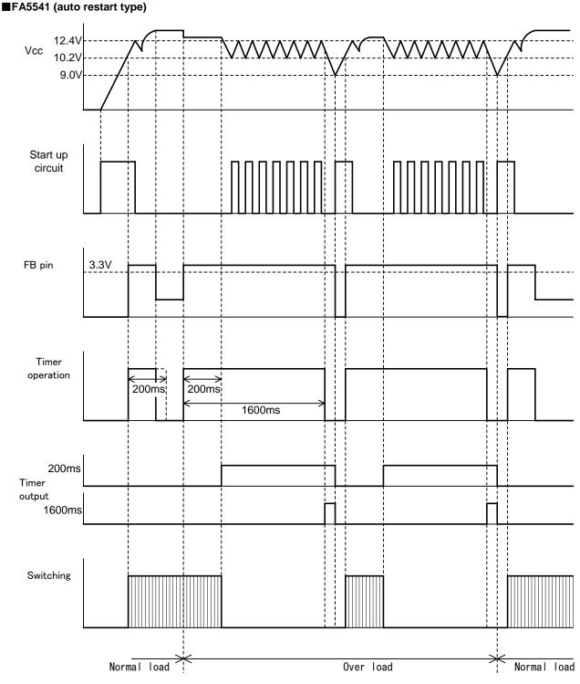
Fig.8 Operation at overload (FA5541)
