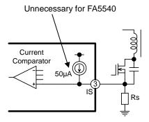
Fig. 16 IS pin circuit
