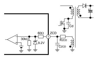
Fig. 10 ZCD pin circuit
