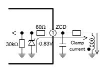
Fig.12 Clamp circuit (negative auxiliary winding voltage)
