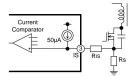
Fig. 17 Filter of IS pin
