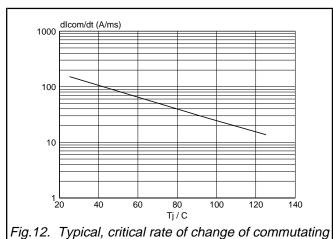
Fig.12. Typical, critical rate of change of commutating current, dl<sub>com</sub>/dt versus junction temperature.
