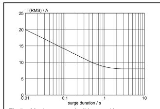
Fig.5. Maximum permissible repetitive rms on-state current  $I_{T(RMS)}$ , versus surge duration, for sinusoidal currents, f = 50 Hz;  $T_{mb} \le 102$ °C.
