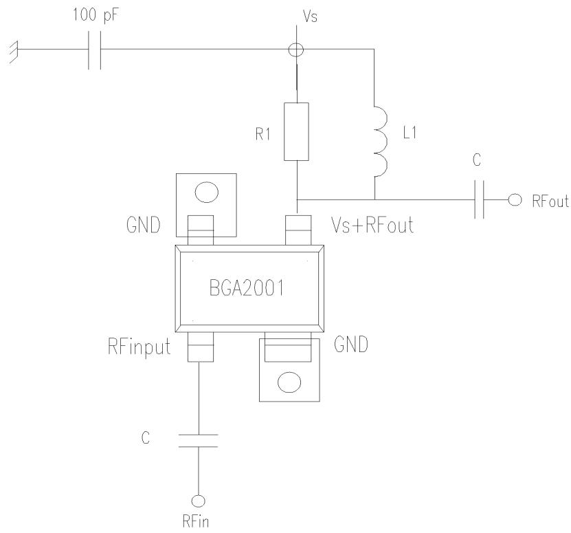
Fig.2 Typical application circuit
