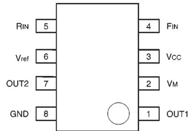
Fig.1 Pin assignments
