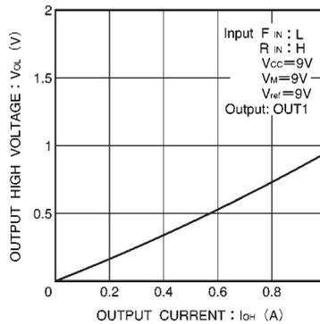
Fig.13 Output low level voltage vs. output current
