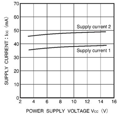
Fig.11 Supply current vs. power supply voltage (BA6417F)
