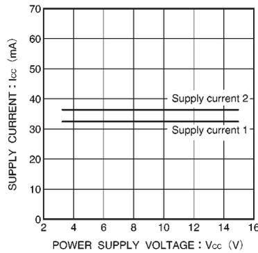
Fig.10 Supply current vs. power supply voltage (BA6289F)
