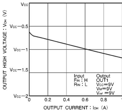
Fig.12 Output high level voltage vs. output current
