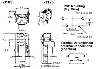
Vertical, Projected Plunger Type (Height: 6.15 mm)
