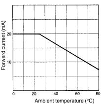
To determine illuminated current of Note: surface illumination types (B3F-9□□□), refer to the above forward current derating curve.
