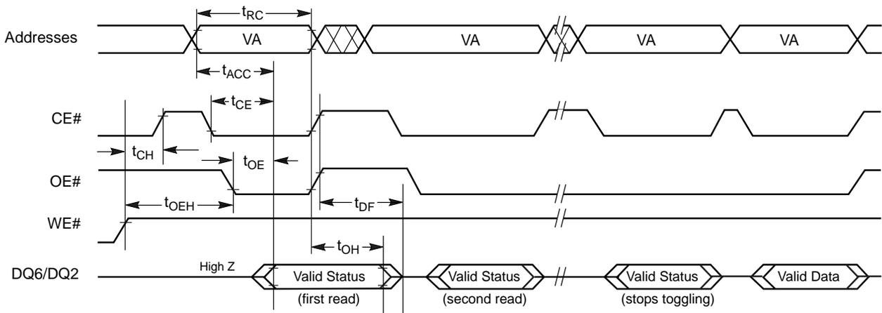
**Note:** VA = Valid address; not required for DQ6. Illustration shows first two status cycle after command sequence, last status read cycle, and array data read cycle.
