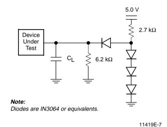
Figure 3. Test Setup
